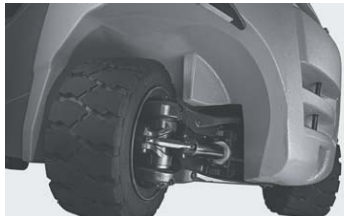
Manoeuvrable and stable high pendulum axle
